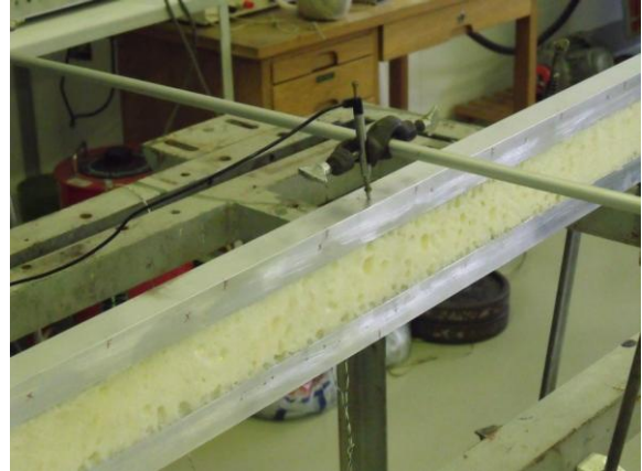
Fig. 5. Measuring of the bending of beam
